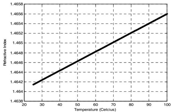
Fig. 5 Effective Refractive Index As A Switch of Temperature in Silica Waveguides
