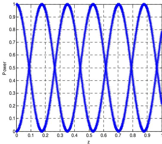
Fig. 4 Power Propagation along  $z$ -direction in Directional Coupler
