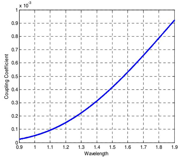
Fig. 3 Coupling Coefficient Characteristic A Function of Wavelength
