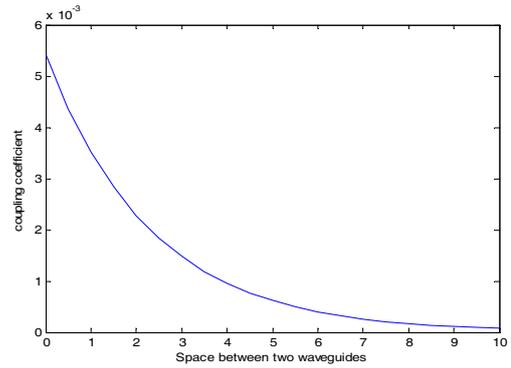
Fig. 2 Characteristic Coupling Coefficient As A Function of Separated Two Waveguides
