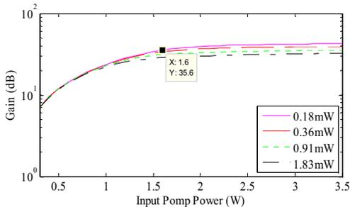
**FIGURE 3.** Variation of amplifier gain with the signal power for several values of the pump power.
