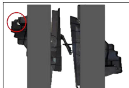
Figure 1 Short shot defects in radiator cover
