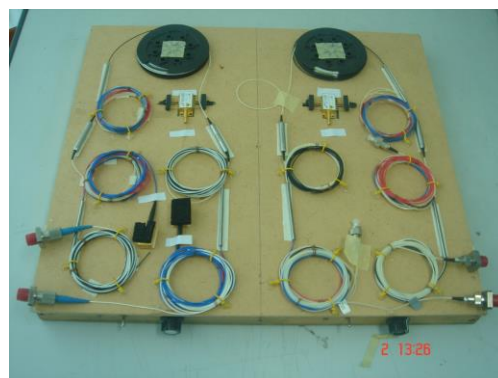
Figure 1. Configuration layout of EDFA experimental setting.
