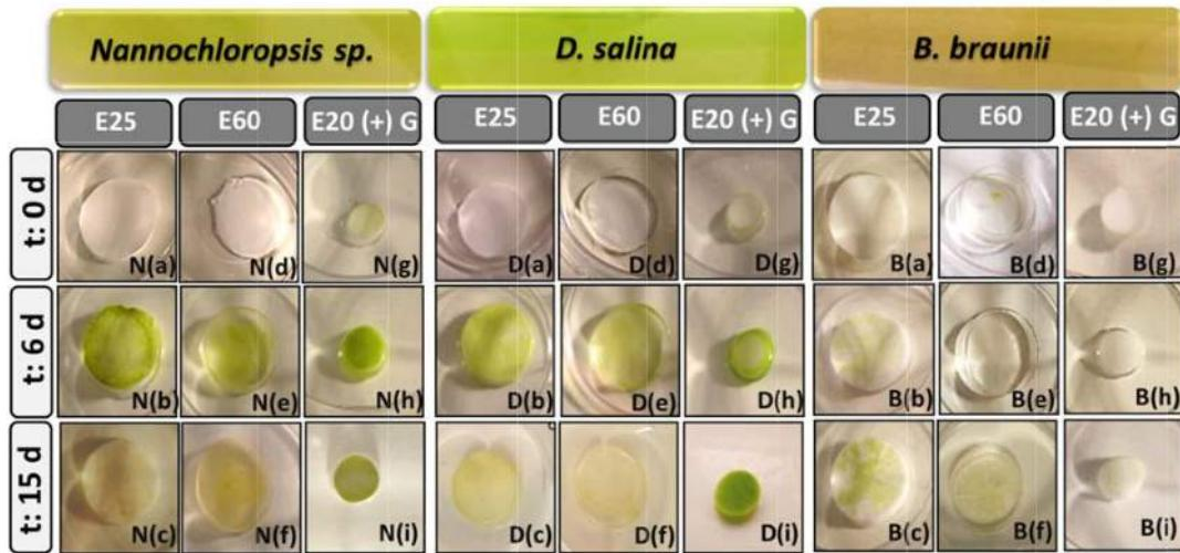
**Figure 4.** Progress of the algal growth on the surfaces of E25, E60 and gelatin-modified E20 PHEMA hydrogel disks (**1<sup>st</sup>-row**) at the beginning, (**2<sup>nd</sup>-row**) after 6 days, and (**3<sup>rd</sup>-row**) after 15 days from the start of the growth experiments. “N” letter represents *Nannochloropsis* sp.; whereas “D” and “B” letters represent *D.salina* and *B.braunii* cells, respectively.
