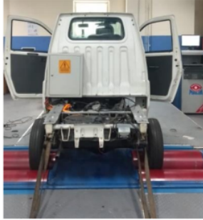
Fig. 5. Performance test on dynamometer
