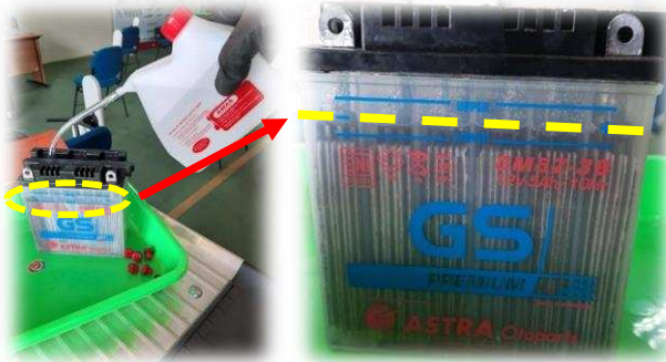
Fig. 5. Lead acid battery
