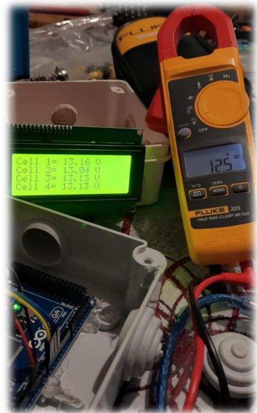
Fig.8. Comparison of voltage measurement by using sensors arrangements and Fluke voltage measurements.
