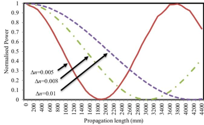
**Figure 4** Power transfer as a function of propagation distance with different refractive index changes.
